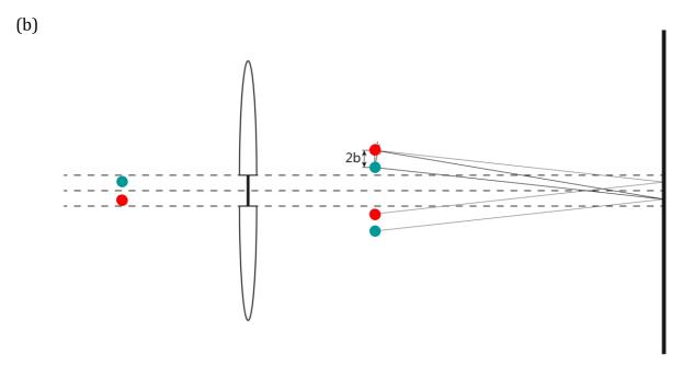
Each source (red or green) will form a pair of images, just like in (a). Each pair forms its own set of interference fringes on the screen. When the red set bright fringes overlap with the dark fringes of the green pair, then the light intensity on the screen is uniform and no fringes can be observed. This means that at any point on the screen, the optical path difference from the red pair should differ from that from the green pair by at least half the wavelength.
